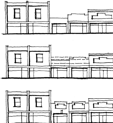
Figure 42 Improving discontinuities in streetscape
